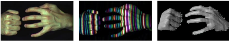
Figure 5.3.: From left to right: two complex physical objects, a pattern of colored straight lines and their deformation when hitting the surfaces, reconstructed 3D shape. From (Zhang et al. 2002).
