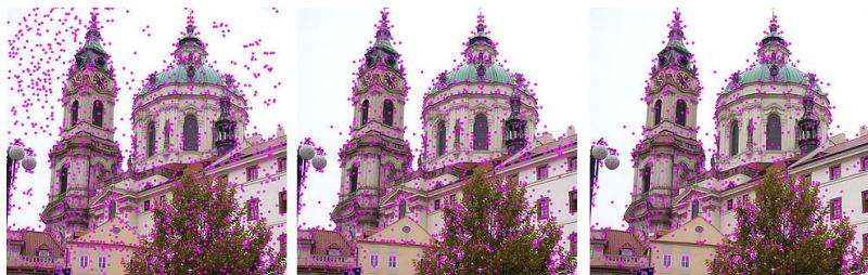
Figure 7.5.: After scale space extrema are detected (left), the SIFT algorithm discards low contrast keypoints (center) and then filters out those located on edges (right). ©Lukas Mach CC-BY 3.0
